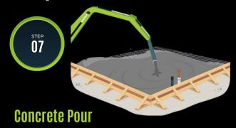
The setup of the concrete pump on site coincides with quality checks on the concrete. Once ready, the concrete is poured, we then follow up with an easy float or a tamp finish.
